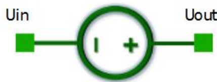
Figure 5.5-8 Voltage source symbol
