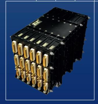
CORECI 2 is a high performance integrated COmpression, REcording and Clphering equipment for high-resolution Earth observation satellites. CORECI 2, in flight since 2021, provides enhanced performance compared to the first generation, whilst maintaining the highest standards of quality and reliability. State of the art performance for onboard data storage, compression and encryption make CORECI 2 the ideal choice for the latest optical Earth observation satellites.
