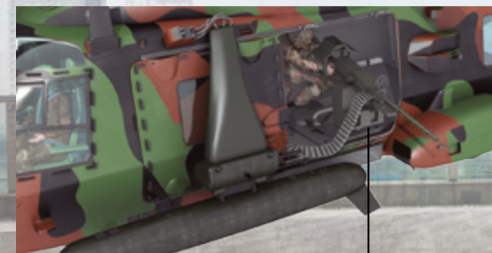
Additional 500 kg external fuel tanks (EAFT) 2 M3M 0.50 machine guns from lateral doors
