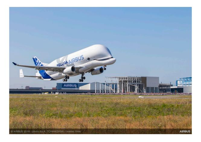
The BelugaXL was launched in November 2014 to address the transport and ramp-up capacity requirements for Airbus beyond 2019. The new oversize air transporters are based on the A330-200 Freighter, with a large re-use of existing components and equipment.
