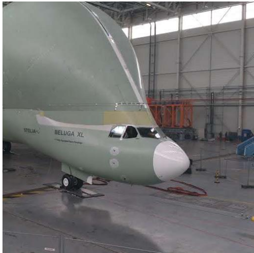
Weighing at 0 degree. Pitch & Longitudinal Centre of Gravity identification
