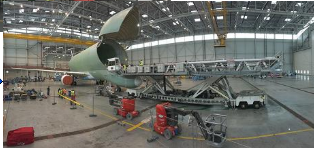
Unloading 8T pallet – first use of Cargo Loader
