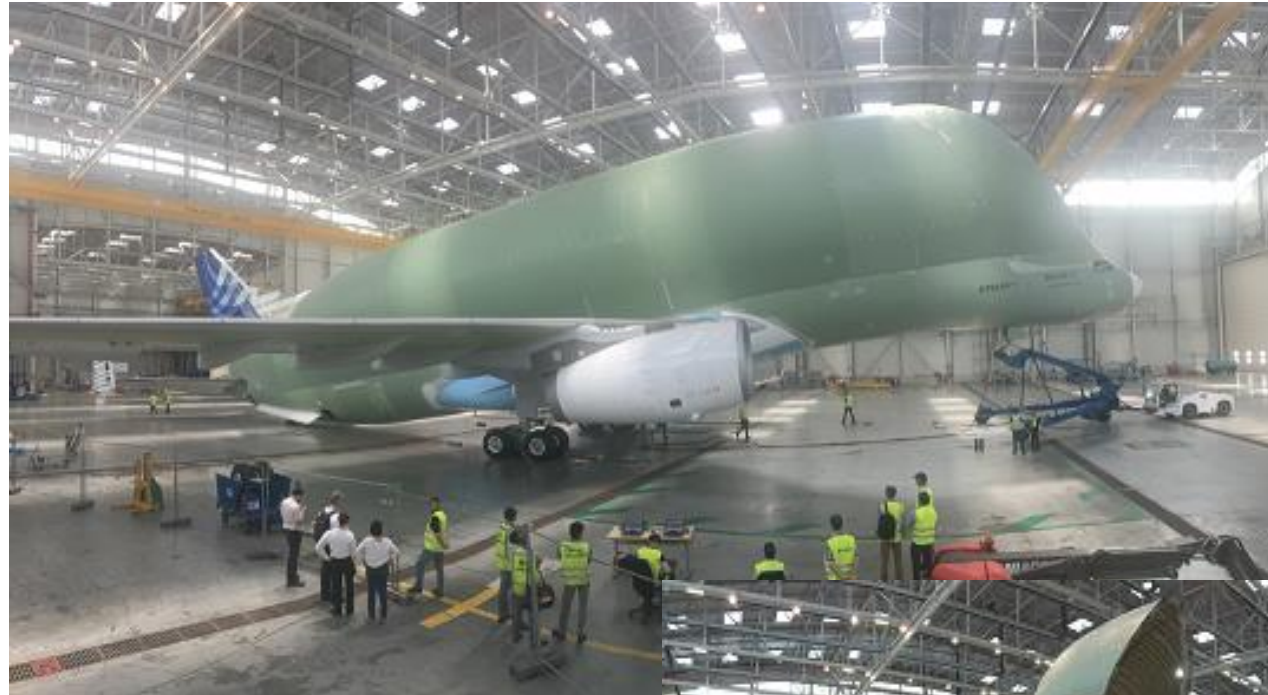
Weighing at 10 degrees. Pitch and Vertical Centre of Gravity identification
