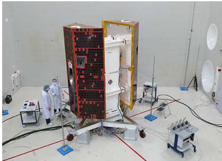
Preparations for the acoustic noise test for the two GRACE-FO satellites, which Airbus constructed for NASA/JPL. Photo: Airbus DS GmbH / Mathias Pikelj
