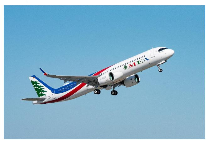
The highly-fuel-efficient A321neo will help reduce MEA's operating costs. The airline's A321neo is powered by Pratt & Whitney's PurePower PW1100G-JM geared turbofan engines and is configured in a comfortable two-class layout with 28 seats in Business and 132 seats in Economy Class and the latest generation in-flight entertainment system and high-speed connectivity.
