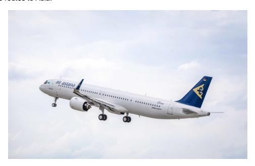
The A321LR is a Long Range (LR) version of the best selling A320neo Family and provides airlines with the flexibility to fly long-range operations of up to 4,000nm (7,400km) and to tap into new long-haul markets, which were not previously accessible with single-aisle aircraft.
