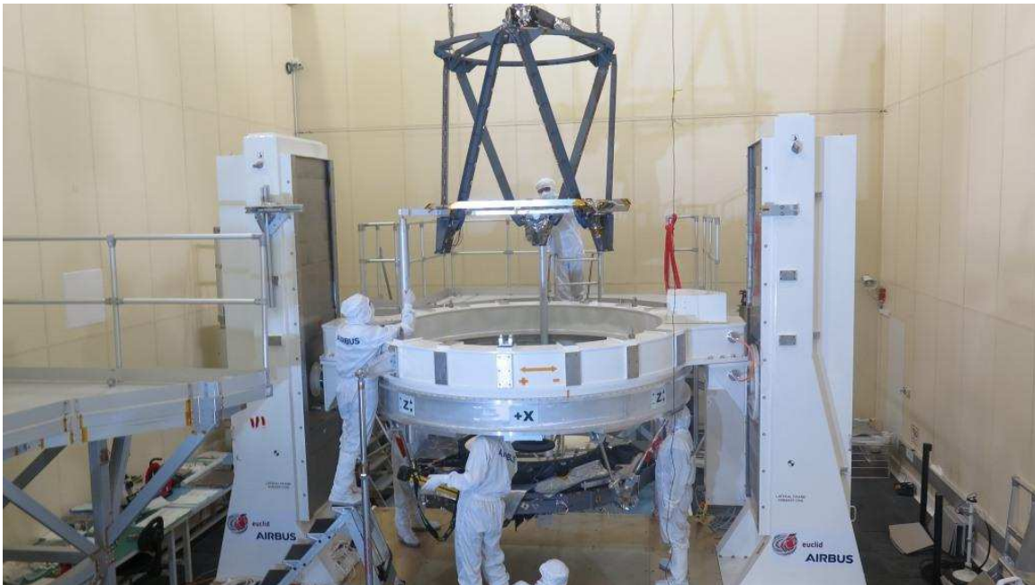
Caption: Euclid's full silicon carbide primary structure
