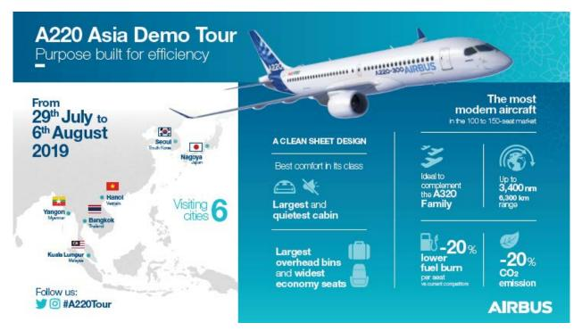
The A220 delivers unbeatable fuel efficiency and true widebody comfort in a single-aisle aircraft. The A220 brings together state-of-the-art aerodynamics, advanced materials and Pratt & Whitney's latest-generation PW1500G geared turbofan engines to offer at least 20 percent lower fuel burn per seat compared to previous generation aircraft. With a range of up to 3,400 nm (6,300 km), the A220 offers the performance of larger single-aisle aircraft.
