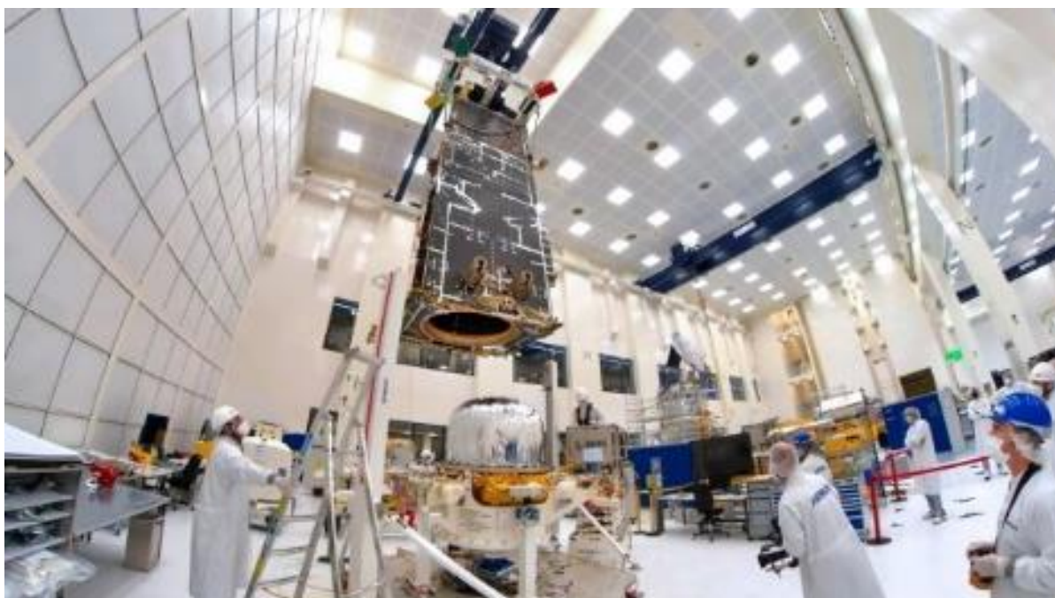
The MetOp-SG B satellite structure being integrated with the propulsion module. Copyright Airbus – M. Pikelj
