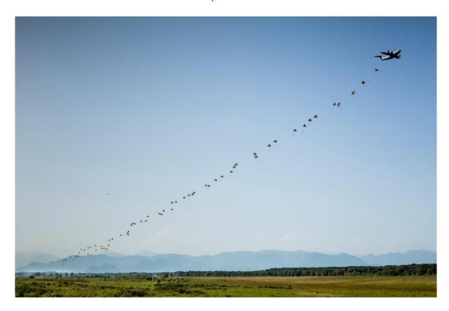
**Getafe, 07 October 2019** – The Airbus A400M new generation airlifter has completed the certification flight test for the simultaneous dispatch of 80 (40+40) equipped paratroopers from both side doors on a single pass. Tests were performed in coordination with the French Armament General Directorate (DGA) together with French and Belgian Armed Forces.
