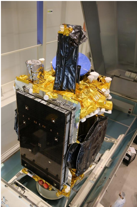
SES-14 is being installed in a travel container
