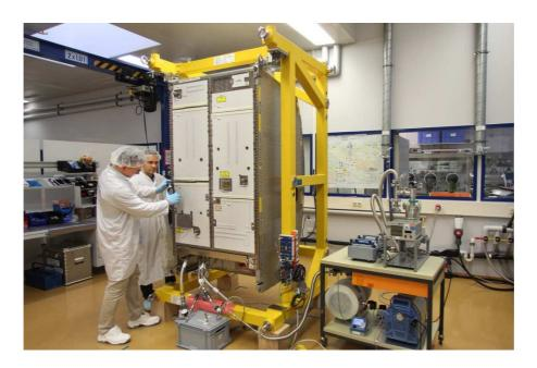
Friedrichshafen, 19/03/2018 – Airbus has delivered the ACLS (Advanced Closed Loop System), an advanced life support system to purify air and produce oxygen for the International Space Station (ISS). The system also produces water, more or less as a by-product of the technology. ACLS was developed by Airbus for the European Space Agency (ESA) and is set to be used as a technology demonstrator on the ISS from summer 2018.
