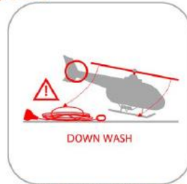
HAZARD - DOWN WASH AND TAIL ROTOR
