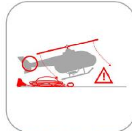
HAZARD - FLAIR LANDING OVER LINES
