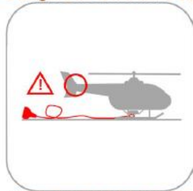
HAZARD - TAIL ROTOR VERSUS LINE LOOPS
