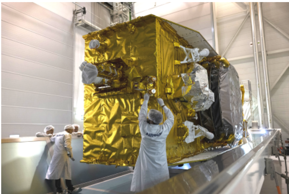
TELEO optical demonstrator hosted on top of Arabsat's Badr-8 satellite - Copyright Airbus
