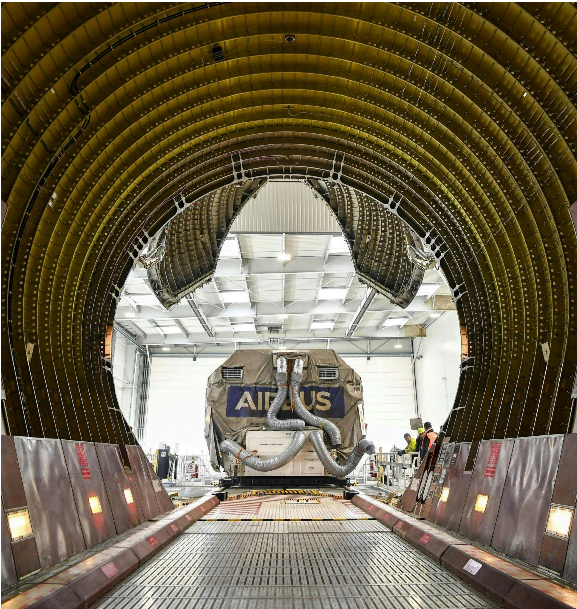
Thuraya 4 satellite container being loaded into the Beluga aircraft - Copyright Airbus
