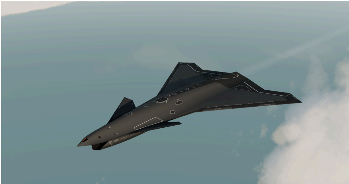
The Wingman is a drone that operates with manned fighter jets and receives its tasks and missions from a pilot in a command aircraft such as the Eurofighter.
