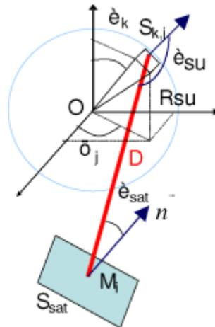
Numerical integration of finite Sun at a finite distance
