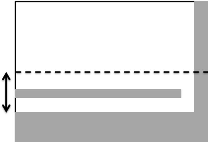
*Exemple of a contact threshold : Even if the two surfaces are close, the lower one will see the cavity, as the rays emitted from this surface will take into account all that is past the Contact Threshold.*
