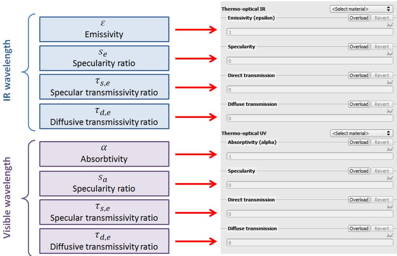
All these coefficients may be defined as incident angle dependent parameters (see figure below). Note that the angle is defined in relation to the tangent to the shape, so that an angle of  $0^\circ$  represents a ray tangent to the surface, and an angle of  $90^\circ$  represents a ray normal to the surface.
