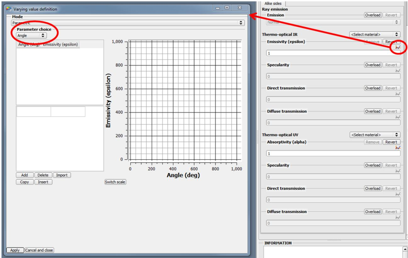
All IR coefficient may otherwise be defined with a wavelength dependency (by selecting "wavelength" for the parameter choice in the figure above). In that case, the wavelength dependent profile may be accurately defined, the wavelength band splitting of the computation being done at processing level.
