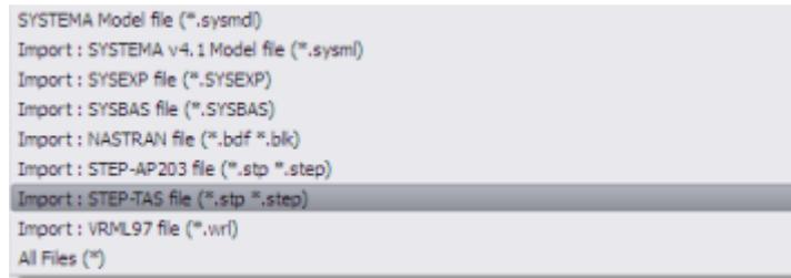
Note that SYSTEMA has an inheritance management which allows setting the properties on a group of object only once. In the case of a STEP-TAS import, all properties are local settings assigned on the shapes. If inherited definitions are preferred, it is the responsibility to the user to make a "delete properties" in a subpart of the model in order to assign the properties only once to the father object.
