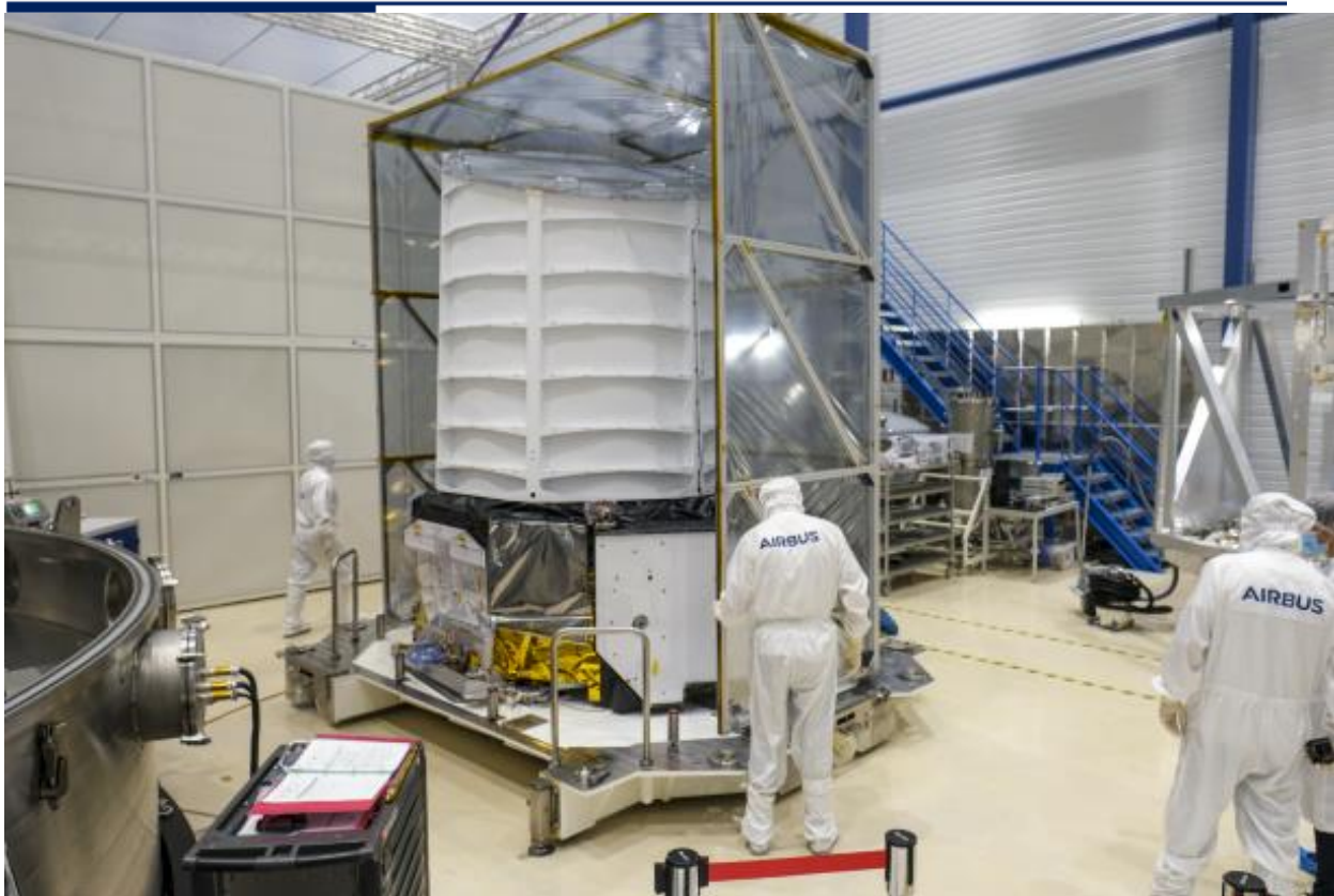
The Airbus-built Telescope for ESA's EUCLID mission being readied for a thermal vacuum test - Copyright Airbus -
