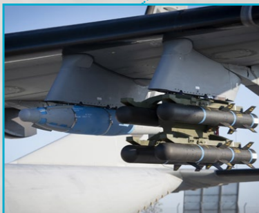
L-UMTAS laser guided anti-tank missile + TEBER-82 laser guidance kit for MK-82 bombs
