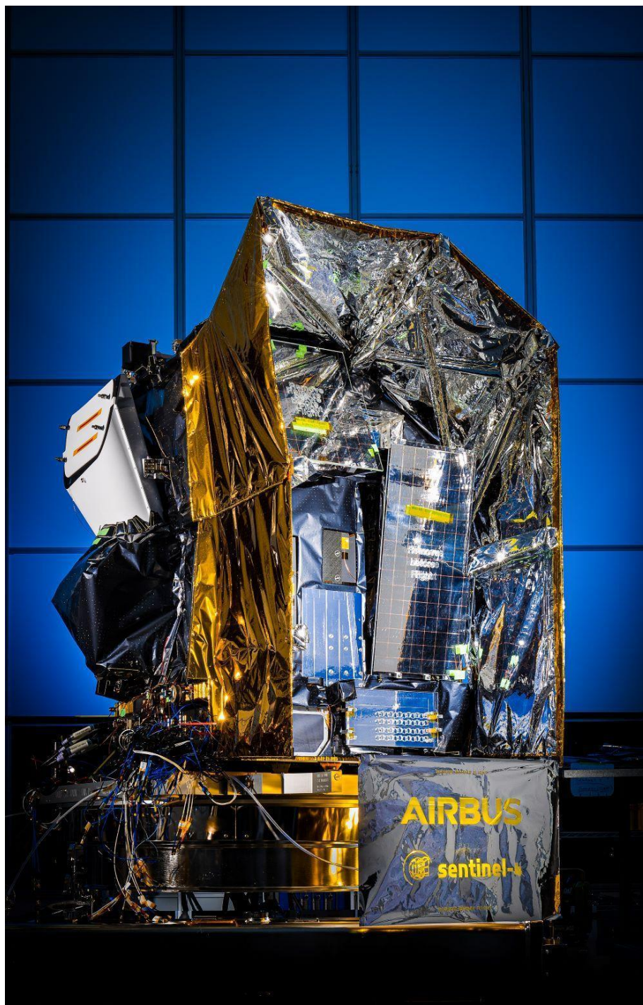
Sentinel-4/UVN air-monitoring instrument flight model - Copyright Airbus 2021 Ralf Maurer
