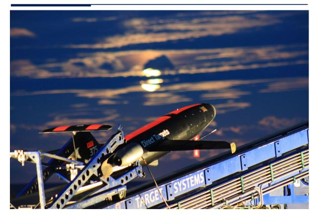
Airbus' 2,000th target display drone simulates fighter jets, drones or cruise missiles that air defenders can engage with live fire to ensure their air defences protect the population in an emergency.
