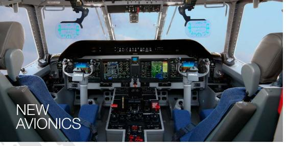
The New C295 is fitted with Collins Aerospace Pro Line Fusion® avionics, delivering a new standard of instrumentation that is ready for the future, compliant with current and forthcoming civil and military requirements. It represents a significant advance in capability for the C295:
