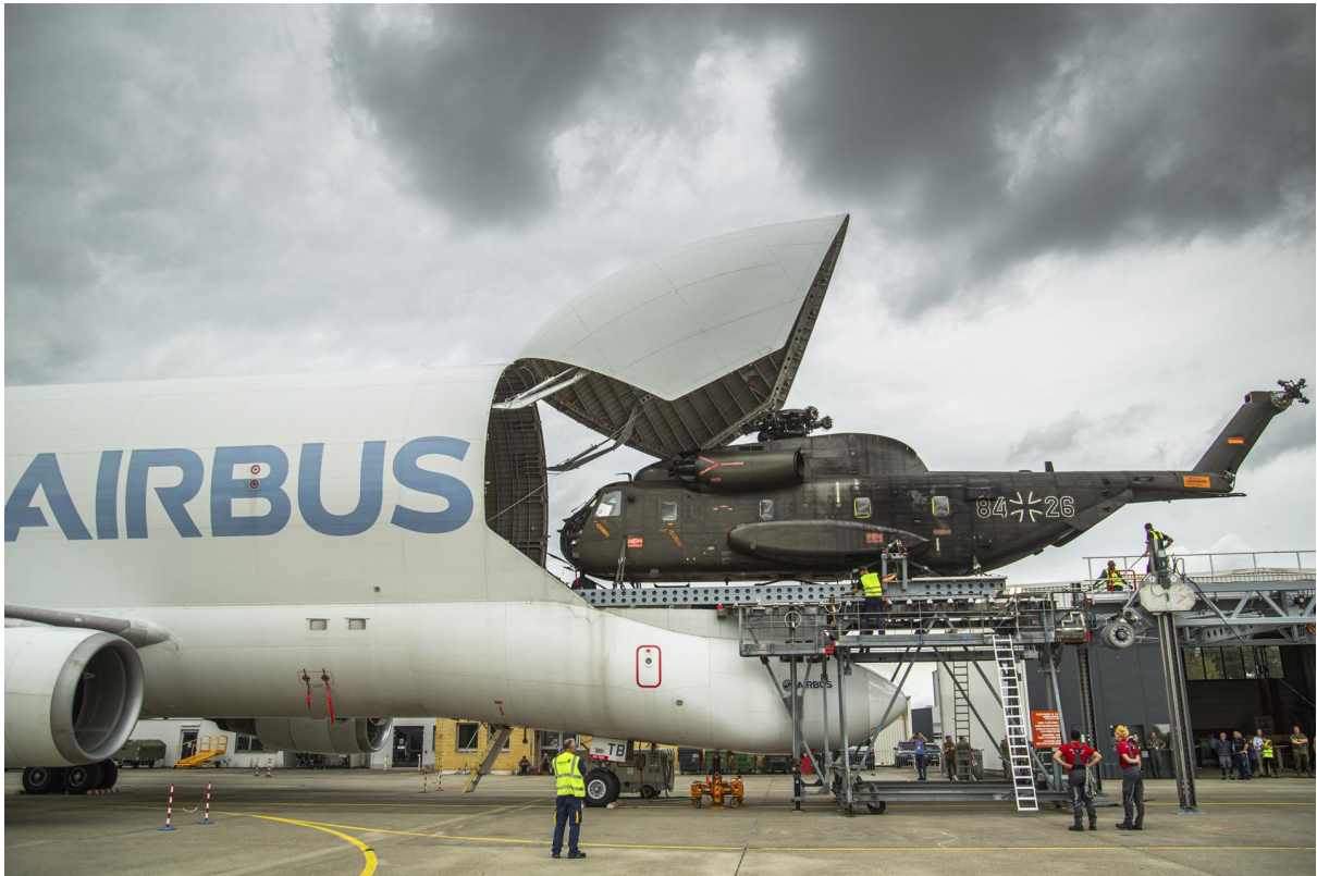
The CH53 helicopter successfully loaded into the Beluga during tests performed at Airbus' Manching site. Copyright: Airbus Defence and Space GmbH 2022.
