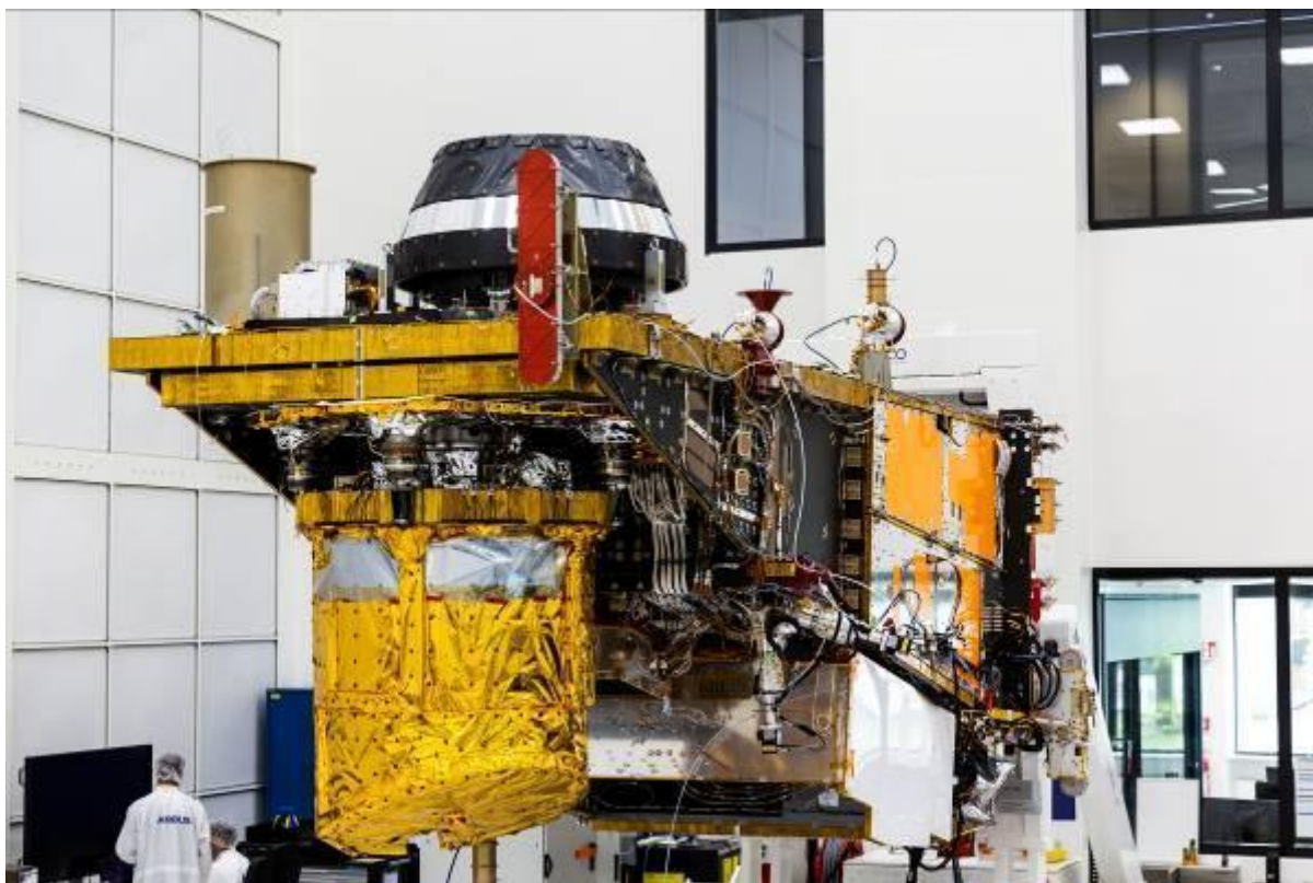
Airbus-built cloud analysing instrument integrated on the MetOp-SG B satellite - Copyright Airbus
