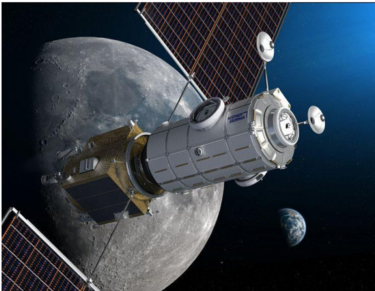
Artist illustration of Northrop Grumman's HALO module and the Power Propulsion Element which form the first critical component of NASA's Gateway.
