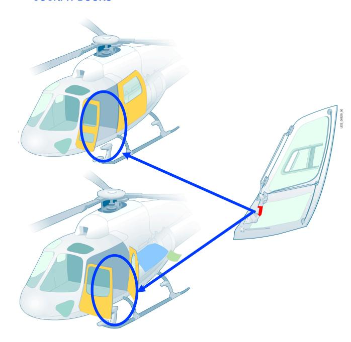
Doors can be jettisoned by actuating the jettison handle. It causes the door to fall away. The handle can be actuated only from the inside
