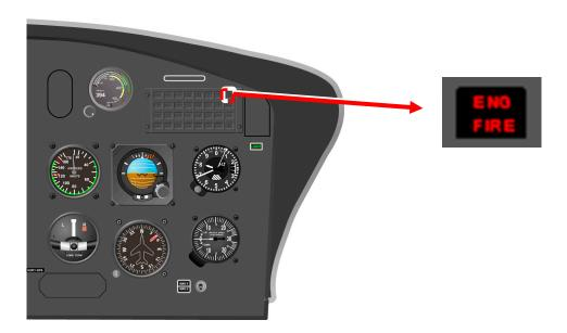
In case of engine fire detection, apply the engine shutdown procedure and refer to the fire in engine compartment paragraph.
