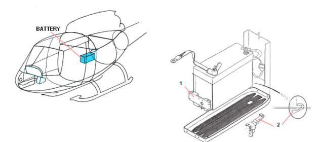
Alkaline type with 20 cadmium-nickel cells.
