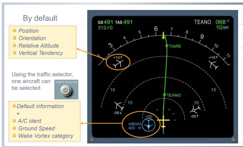
“The A330neo cockpit also features ‘**Autopilot / Flight Director Traffic Collision Avoidance System**’ (AP/FD TCAS) mode. This is an enhancement whose timeline is associated with these new airliners. So for pilots in an A330neo, if they have traffic venturing close, then the automation can help them to proactively avoid it. The resolving manoeuvre
