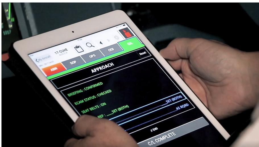
Willey points out: “With these interactive checklists you can quickly determine from the colour-codes which items have been completed versus those not yet done. This reduces the chance of missing a step, say, if the process has been interrupted for any reason.”
