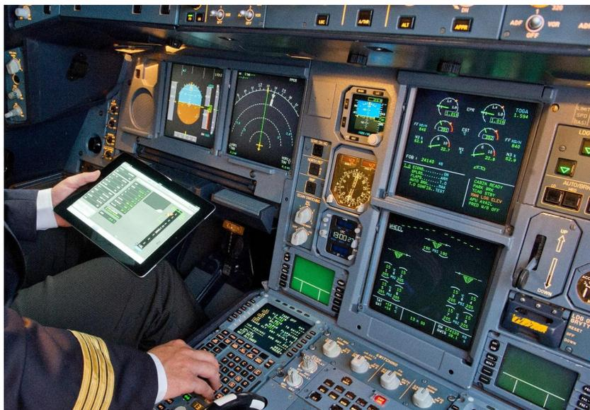
“The FOMAX router is a very big step forward allowing A330neo pilots to communicate with the open world and with the aircraft avionics (as they can on the A350 using its docking station), however in this case by connecting their hand-held (or dashboard mounted) EFBs via wi-fi.”
