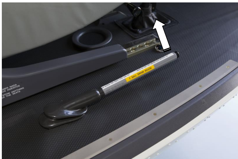
For activation press button on front of the lever and pull
