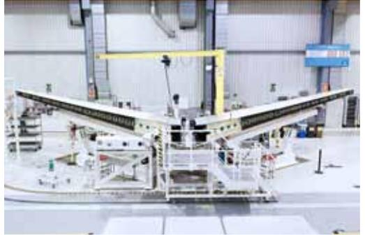
Using composites in the fuselage and the wing also reduces the need for fatigue-related inspections that are required on traditional airliners built with aluminium. The composites and titanium also reduce the need for corrosion-related checks. All three aircraft in the A350 XWB family will share the same wing platform, which is built primarily from carbon composite materials.
