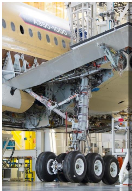
First new 6 wheel bogie Main Landing Gear fitted on the MSN59
