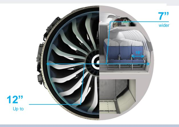
A320 Improved engines Higher by pass ratio 12:1 Higher EGT margin Lower engine DMC cost
