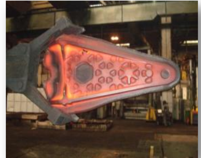
Pylon Pyramid – Forging
