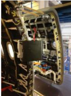
CFRP Doors Surrounding structure - Barrel 1B
