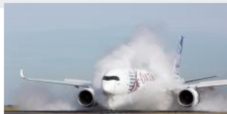
Water ingestion test at Istres MSN004, May-9th 2014
