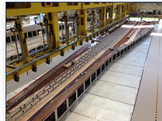
Stringers positioned in Wing Upper Cover // Stade
