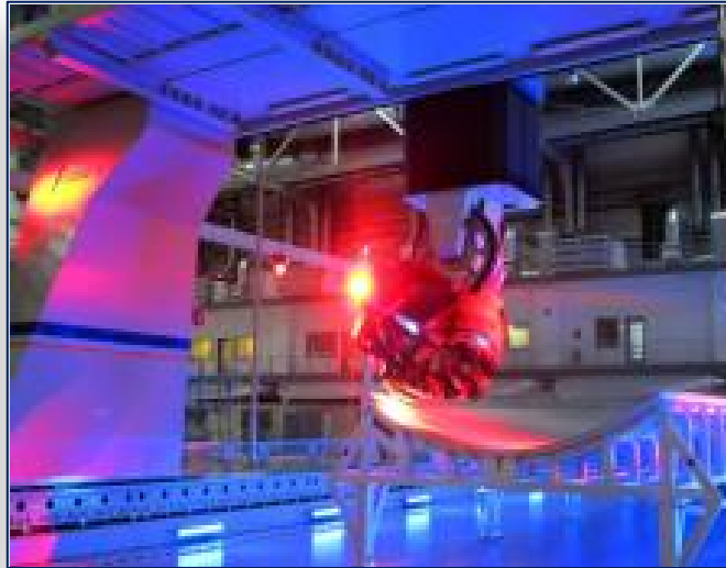
PAG CFRP S13/14 Fuselage shell – 1 st Ply
