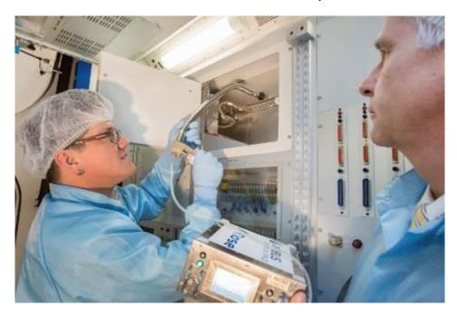
The new, trunk-like instrument of the 'E-nose' can detect micro-bacterial contamination in every corner of the Space Station. Viktor Fetter (left) and Thomas Hummel from Airbus Defence and Space take samples in an ISS ground module.
