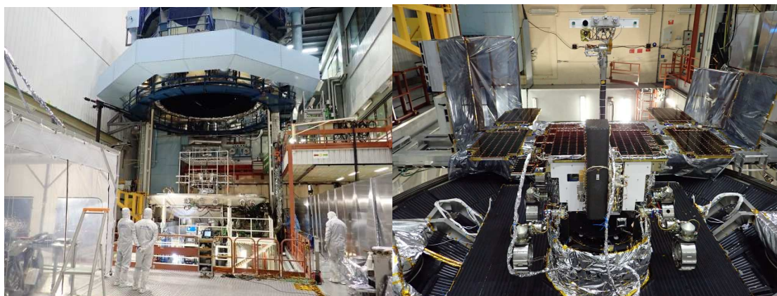
Thermal-vacuum testing for ExoMars at Airbus in Toulouse © Airbus
