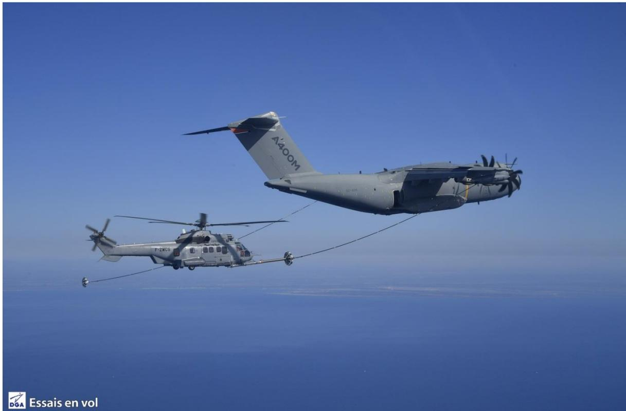
**Getafe, 24 September 2019** – The Airbus A400M new generation airlifter has successfully achieved its first helicopter air-to-air refueling contacts with an H225M. Over the course of 4 flights, operated in day conditions over the south of France, the A400M performed 51 dry contacts marking a decisive milestone towards its full capability as a tanker. These tests were performed under the coordination of the French “DGA Essais en vol” flight test centre.
