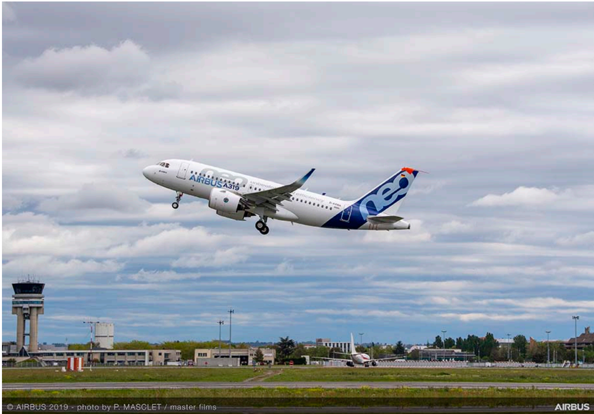
The A319neo prototype takes off from Toulouse with its new P&W GTF engines.
