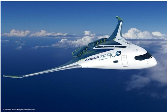
**A “blended-wing body” design** (up to 200 passengers) concept in which the wings merge with the main body of the aircraft with a range similar to that of the turbofan concept. The exceptionally wide fuselage opens up multiple options for hydrogen storage and distribution, and for cabin layout.
