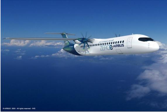
**A turboprop design** (up to 100 passengers) using a turboprop engine instead of a turbofan and also powered by hydrogen combustion in modified gas-turbine engines, which would be capable of traveling more than 1,000 nautical miles, making it a perfect option for short-haul trips.
