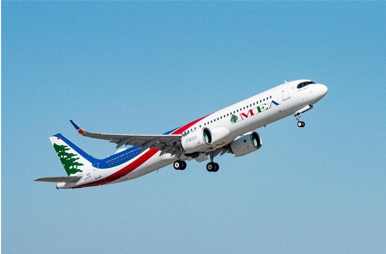
The highly-fuel-efficient A321neo will help reduce MEA's operating costs. The airline's A321neo is powered by Pratt & Whitney's PurePower PW1100G-JM geared turbofan engines and is configured in a comfortable two-class layout with 28 seats in Business and 132 seats in Economy Class and the latest generation in-flight entertainment system and high-speed connectivity.
