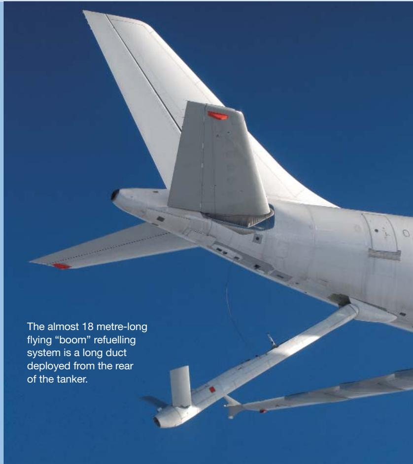
The almost 18 metre-long flying "boom" refuelling system is a long duct deployed from the rear of the tanker.
