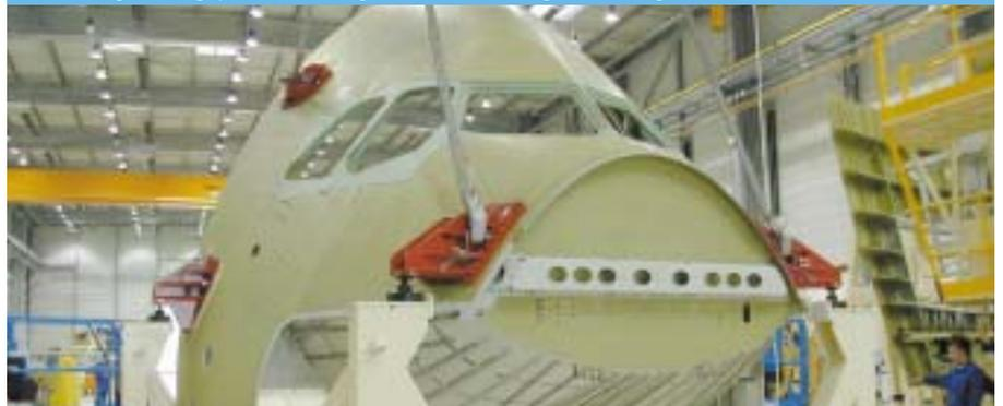
Méaulte plant in France produces the A380 particularly impressive nose section. The first delivery was on November, 23.
