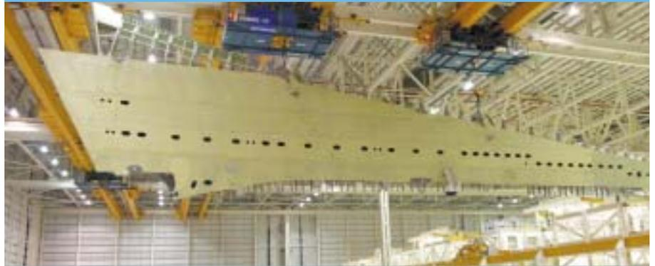
At 36.3m long, the wings produced in Broughton in UK are the largest-ever designed and built for a commercial aircraft.
