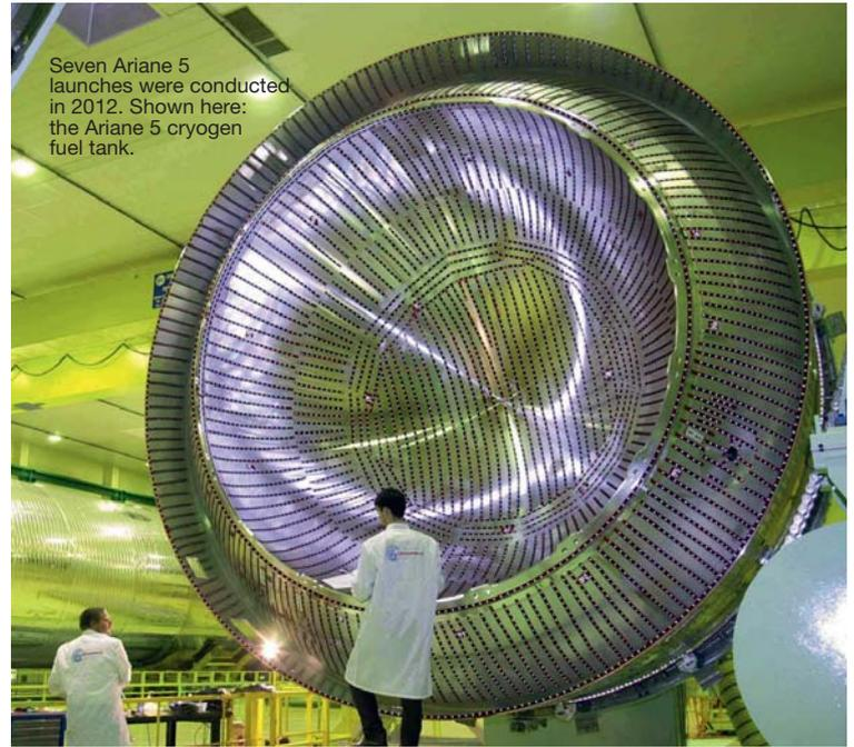
Seven Ariane 5 launches were conducted in 2012. Shown here: the Ariane 5 cryogenic fuel tank.
