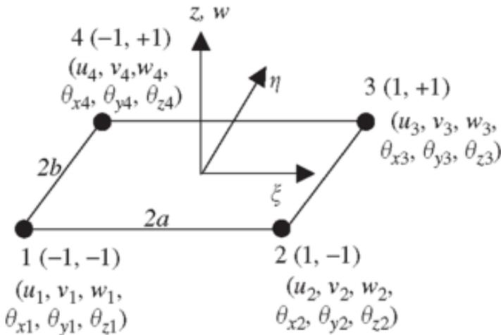
The vector of displacements for the single node “1” is in this case:
