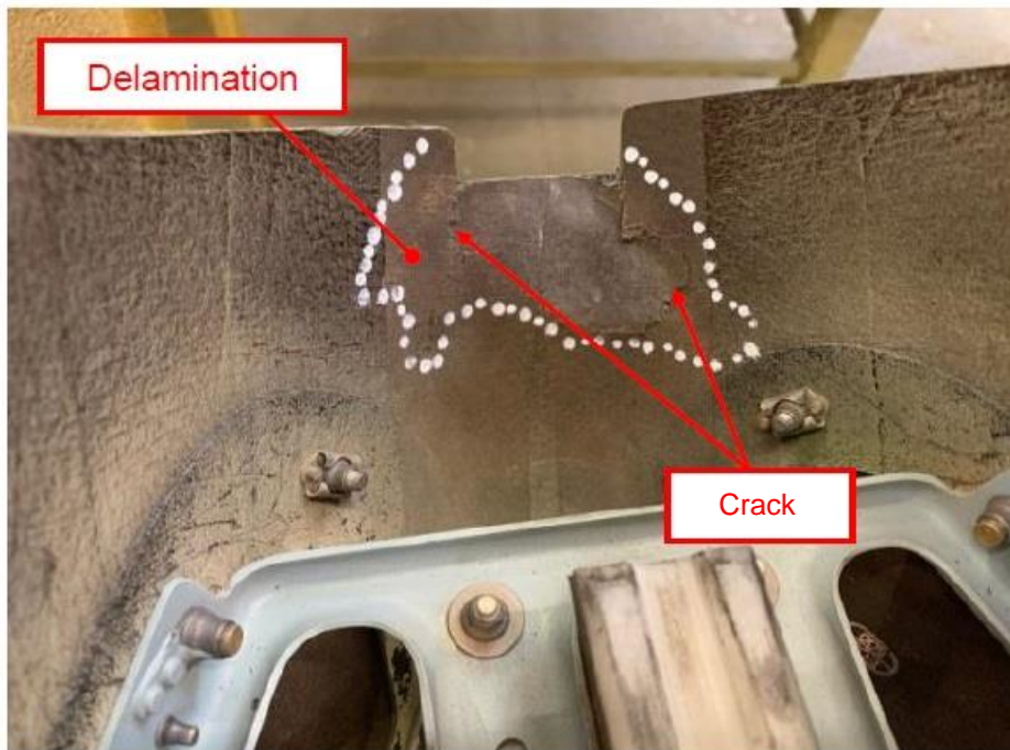
Figure 13: Delamination on cowling with crack
