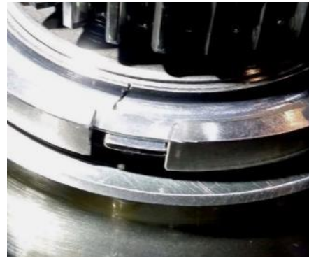
Figure 6: Crack (nut retainer bush)
