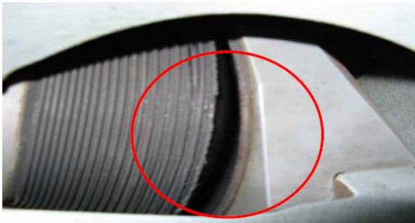
Figure 10: Partial delamination of the elastomer
