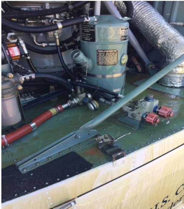
Figure 16: Example of fluid leak or seepage on the transmission deck with overflow on the fuselage.
