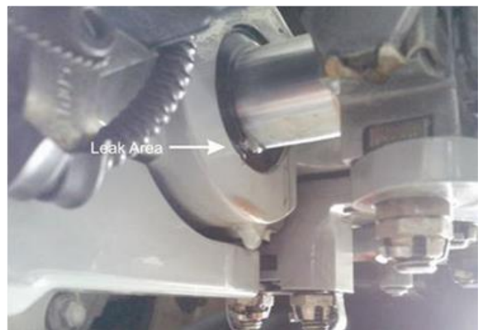
Figure 16: Example of fluid leak or seepage on the transmission deck with overflow on the fuselage.
