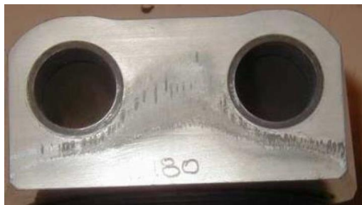
Figure 7: Fretting (spherical thrust bearing)
