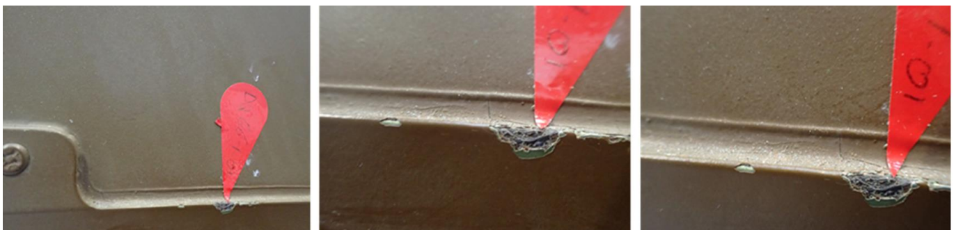
Figure 14: Impact on composite structure
