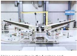
Using composites in the fuselage and the wing also reduces the need for fatigue-related inspections that are required on traditional airliners built with aluminium. The composites and titanium also reduce the need for corrosion-related checks. All three aircraft in the A350 XWB family will share the same wing platform, which is built primarily from carbon composite materials.
